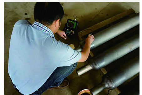
Radiant tube UT inspection
