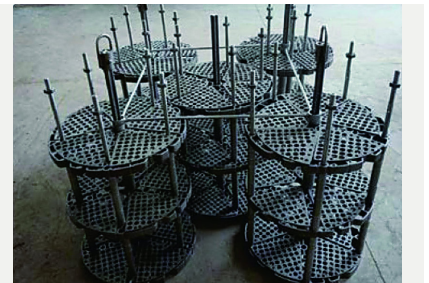
Loading system for pit furnaces
