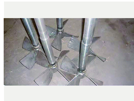
Fan blades for mesh belt furnaces
