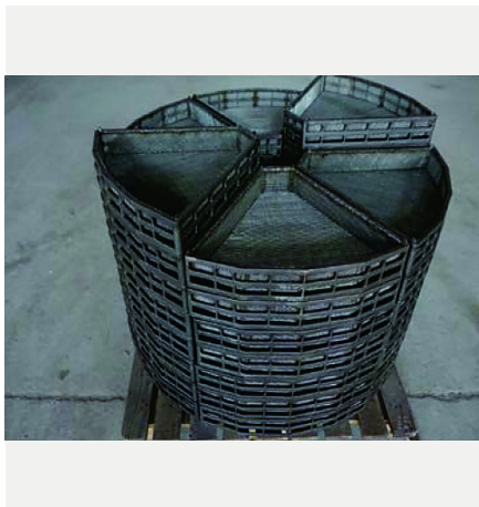
Loading fixture for pit furnaces
