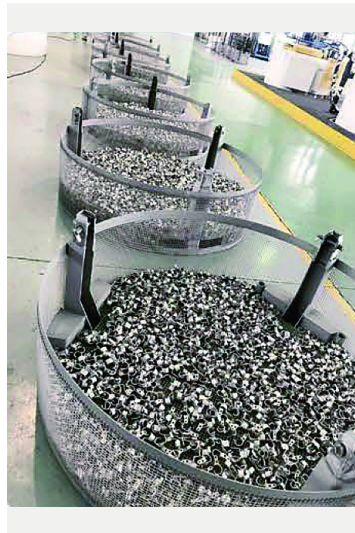
Welding fixtures for nitriding furnaces
