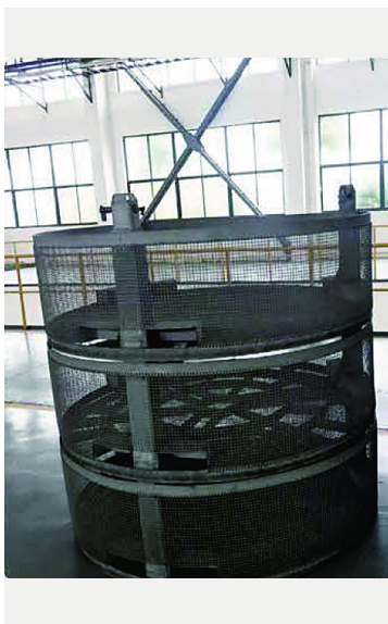
Welding fixtures for nitriding furnaces
