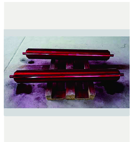
PT inspection for rollers
