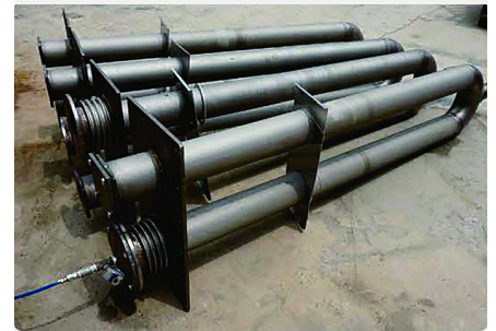
Radiant tube pressure test
