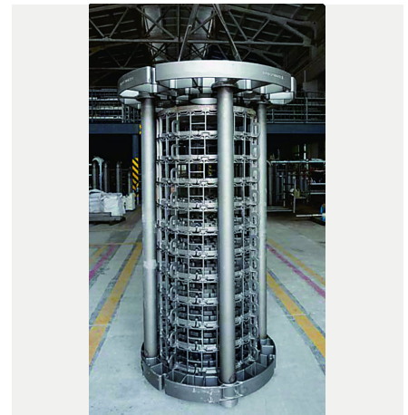
Loading system for pit furnaces
