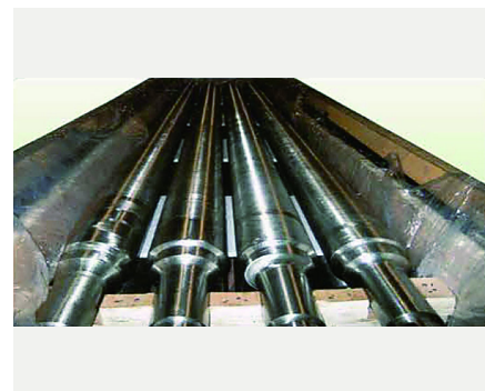
Industrial furnace rollers
